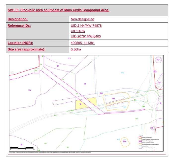
A proposed stockpile area located between the existing A303 and the temporary road to Winterbourne Stoke crossroads. The site is bisected by a utility corridor (Site 49).
