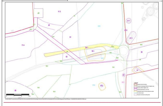
Site 54 is a short linear corridor north of the existing A303. During construction, a temporary road would carry traffic between the northern dumb-bell roundabout and the existing Winterbourne Stoke Crossroads roundabout. In order to construct the temporary road at the eastern end a small wooded area will be cleared of vegetation.
